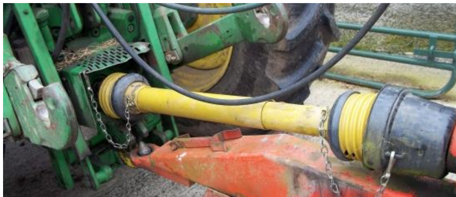
Operate PTO shaft with guard properly fitted
