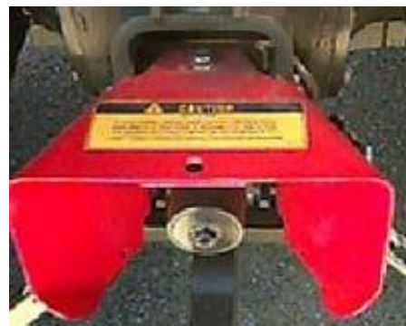
Keep PTO master shield in position
